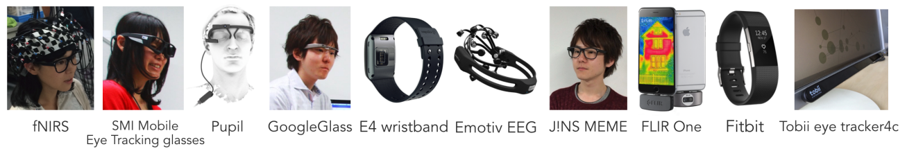
Figure 1. Examples of sensors in this research field sorted by their pervasiveness (left: advanced but expensive; right: inexpensive)
