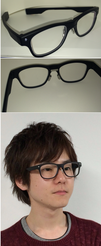
Figure 1: The EOG Glasses used for the experiments. The second picture shows the 3 electrodes touching each side of the nose and the area between the eyes. The last picture shows a user wearing JINS MEME.
